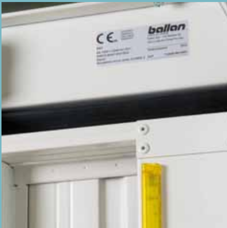
CE product identification dataplate stating all the data required by current statutory regulations.
