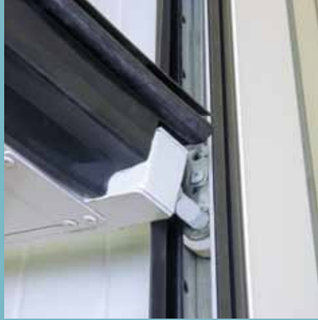
Cable break device incorporated in the vertical tracks: engages in the event of cable breakage to prevent the door leaf from dropping.
