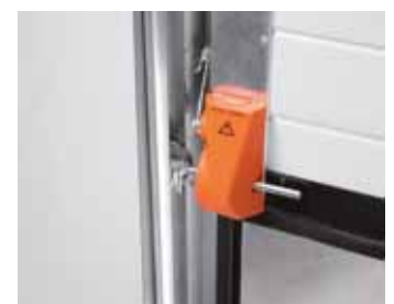
Cable break device that engages in the event of cable breakage that instantly stops the door from closing (optional).
