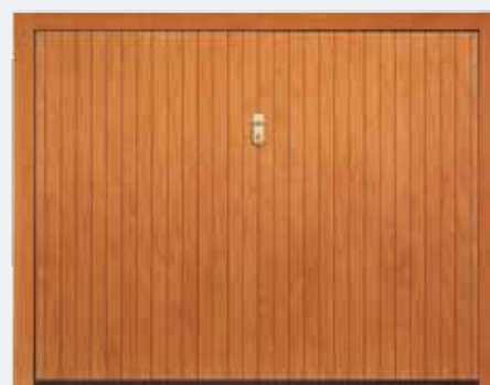
External view of Reserve Sikura HF up-and-over door, covered with multi-ply okoumé and outer cladding in oak decorated by pantograph with horizontal slats with an 85 mm pitch. The outer cladding in oak, full treatment with colour 1 and the lock with Defender art. 94 are optional.
